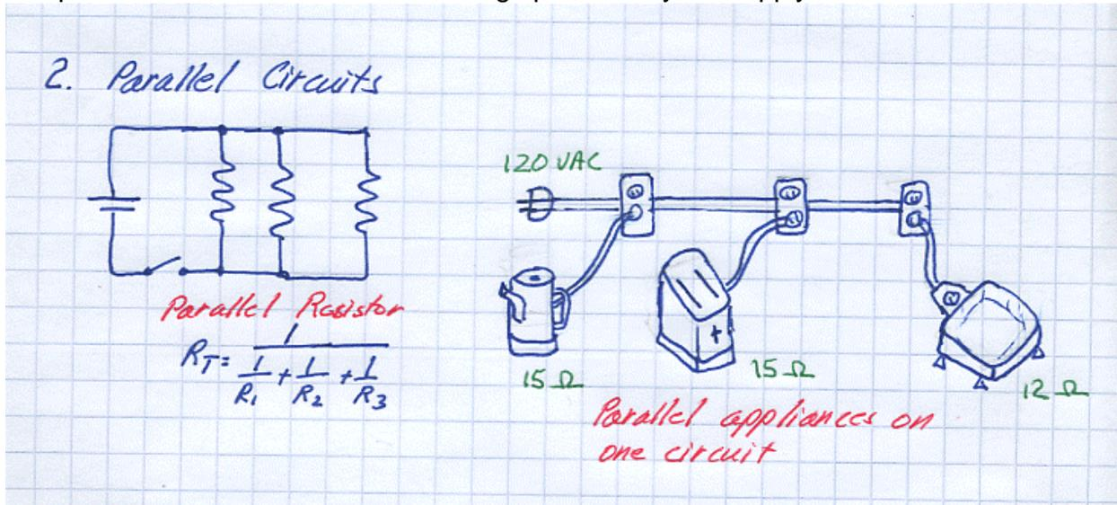
2. When the resistances are connected in parallel, the total resistance ( $R_T$ ) in the circuit is less than the resistor with the least value. The formulas for solving for total parallel resistance are:
