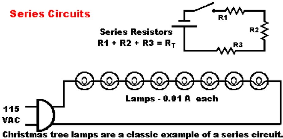
2. When the **resistances are connected in series**, the total resistance ( $R_T$ ) in the circuit is equal to **the sum of the resistances of all the paths** of the circuit. The formula for solving for total series resistance is:
