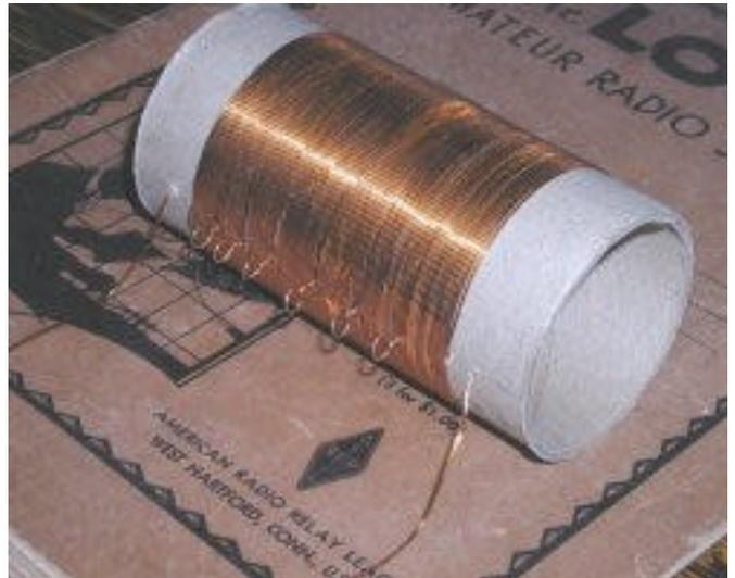
The coil below uses 60 turns of #18 plastic coated stranded wire wound on a mailing tube with a 4.2” outside diameter. The taps are at turns number 5, 10, 15, 30, and 45. The plastic-coated wire is not as stiff as the enamel wire so a wood dowel is used as an aid for tap formation. Use this number for inductance in addition to the capacitance to solve for the tuning range of your radio.
