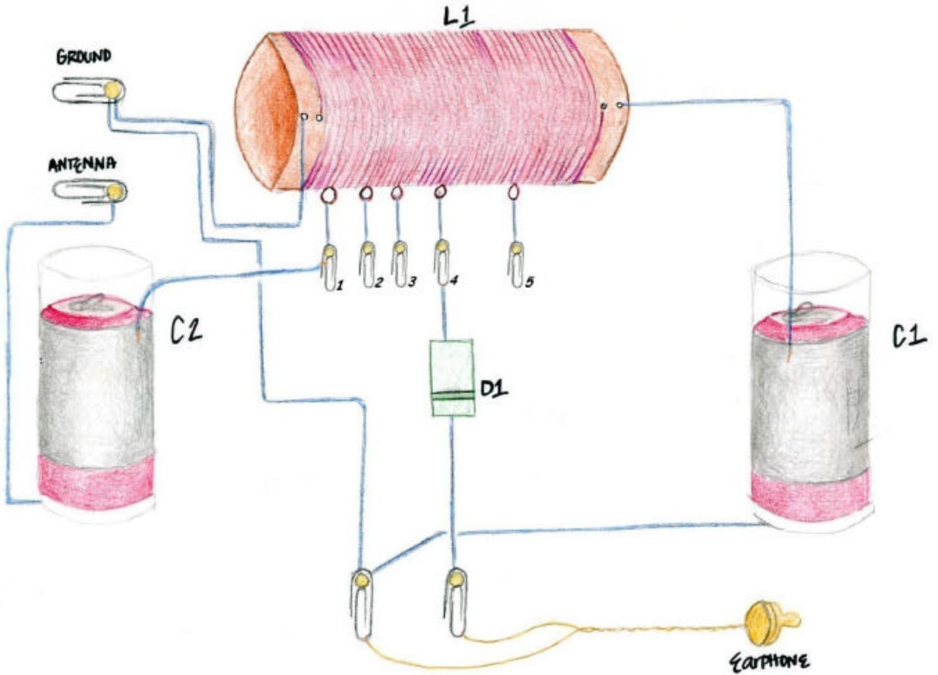
The above is a pictorial diagram of the crystal radio to show the approximate physical placement of the components.
